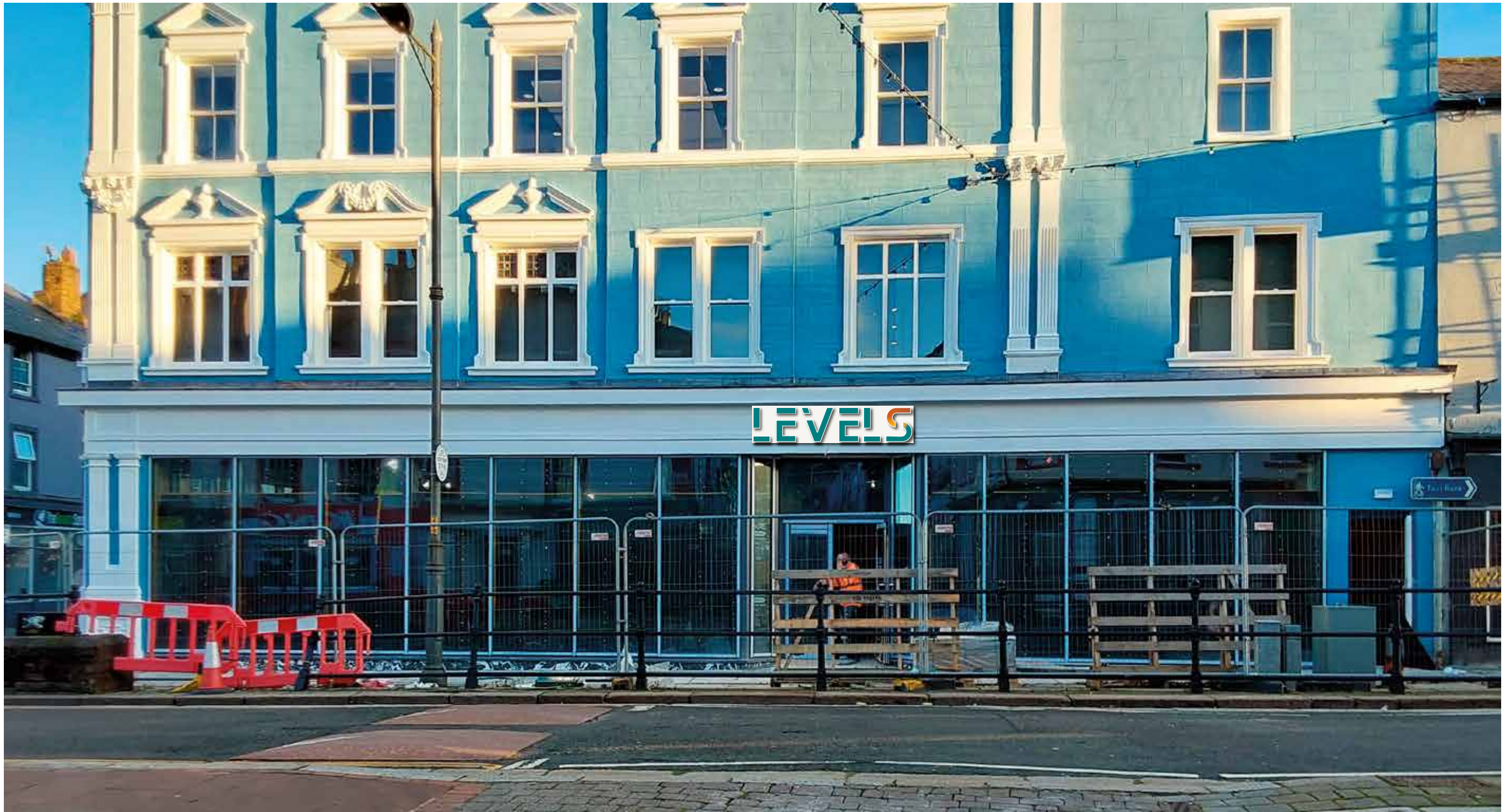
ITEM A 2350mm (w) x 512mm (h) Built up letters fitted onto signtray with 50mm returns 2390mm (w) x 55mm (h)
